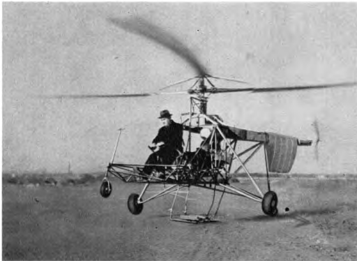
4. America's first successful helicopter, the Sikorsky VS-300 of 1939 brought answers to problems which so long had been unsolved. It could fly up, backward, sideways, forward, in circles or hover for sustained periods. Its full controllability opened a bright new chapter in world aviation.
